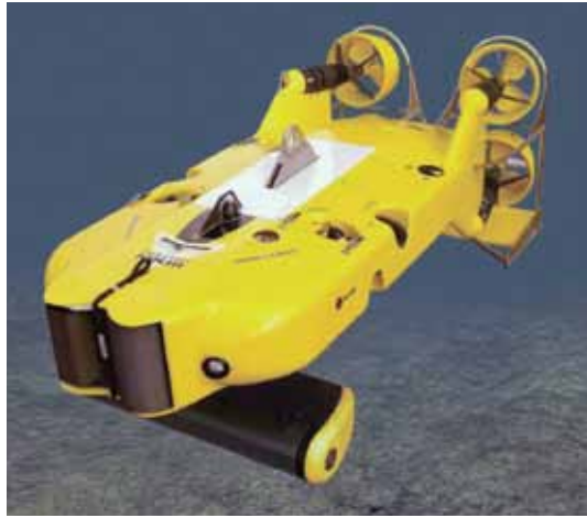
Double Eagle MK-III UUV, built by Saab for tethered or autonomous operation, is used by the Australian, Canadian, Swedish, and other navies. Its principal mission is MCM operations.
