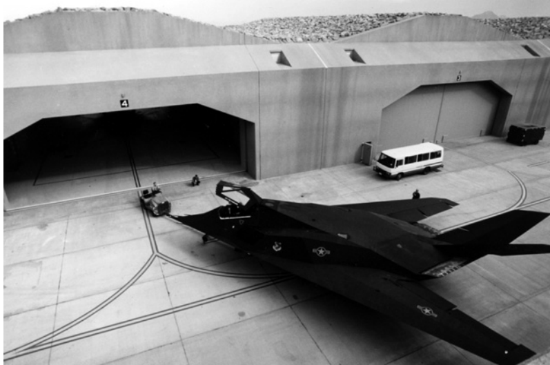
Figure 4.1—F-117 Fighter Being Towed into a Concrete Hardened Aircraft Shelter
