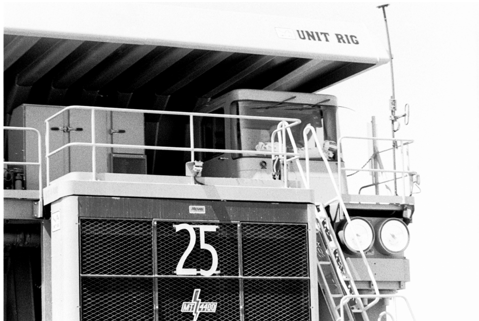
A video camera mounted on the front of a haul truck at a mine helps drivers see personnel and equipment in their vicinity.
