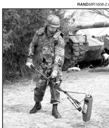
Figure 2.8—Nomadics' Sensor for Detecting Explosive Vapors
