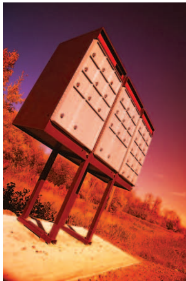
Figure 3.1 Cluster-Box Units, One Type of Multiple-Mailbox Delivery Point
