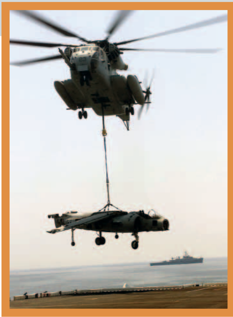
A CH-53 Sea Stallion, a current heavy-lift platform, drops a retired AV-8 Harrier on the flight deck of the USS Saipan (LHA 2).
