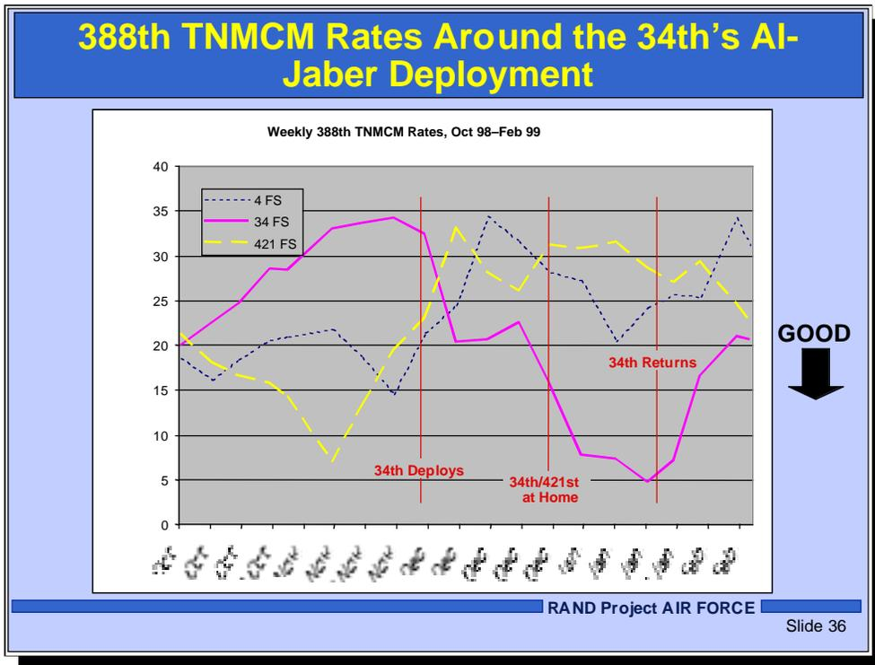
TNMCM rates mirror the MC rates to a large extent. Notably, the 34th's TNMCM rates rise strongly in the weeks before the deployment, signaling that the squadron was focusing on getting the deploying jets ready at the expense of the jets being left at home station. And, during the final week or two, the rates for the other two squadrons jump because their maintainers are helping the 34th ready the deploying jets while the 34th's maintainers prepare themselves to deploy.
