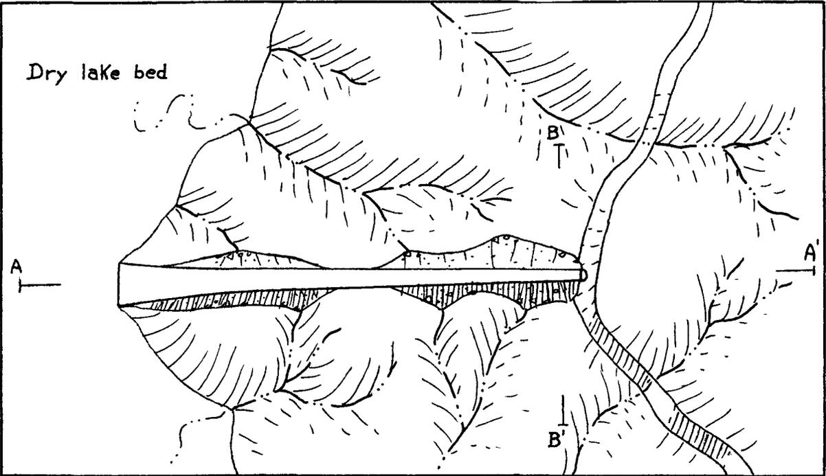
Figure 4 Map view of proposed entrance ramp and tunnel design.
