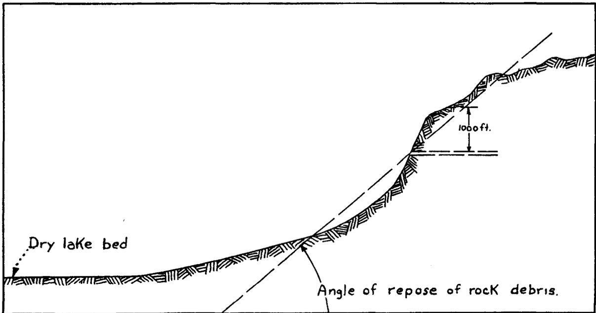
Figure 3 Vertical section through an ideal mountain slope.
