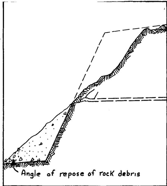
Figure 2 Vertical section showing blocked tunnel.
