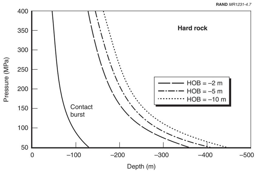
**Figure 4.7—Peak Overpressure Versus Depth for 100-kT Warhead**
