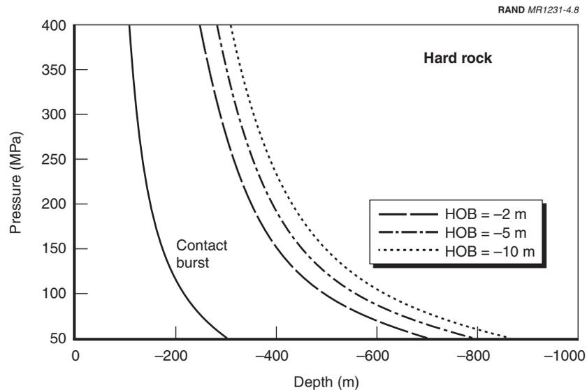
Figure 4.8—Peak Overpressure Versus Depth for 1000-kT Warhead
