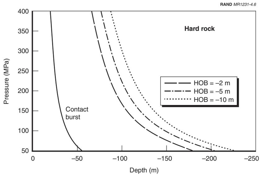
**Figure 4.6—Peak Overpressure Versus Depth for 10-kT Warhead**
