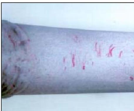
**Figure 12b: Crazed Cracking**
