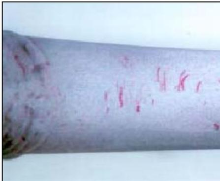
**Figure A1b: Crazed Cracking**
