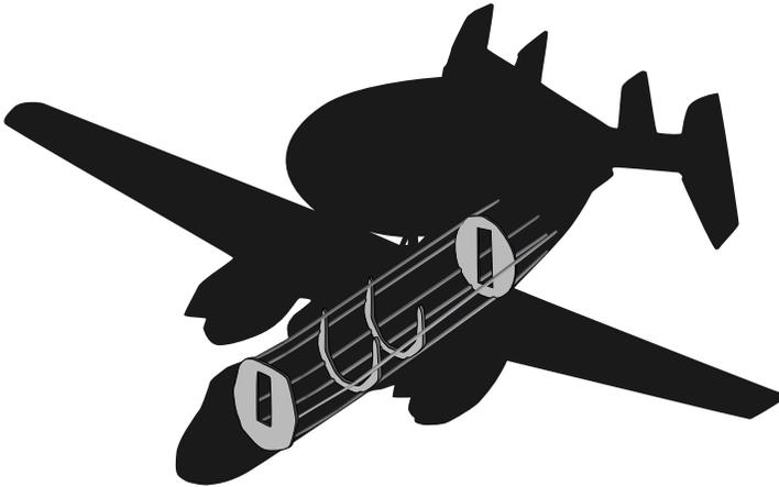
Figure 3.1—Sections of Aircraft Modified to Accommodate RMP Avionics
