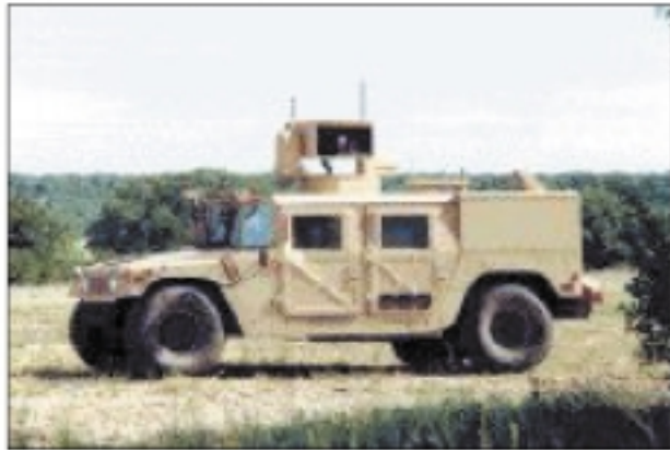
Figure D.1—HMMWV-Based UGV Used in DARPA Demo II Program
