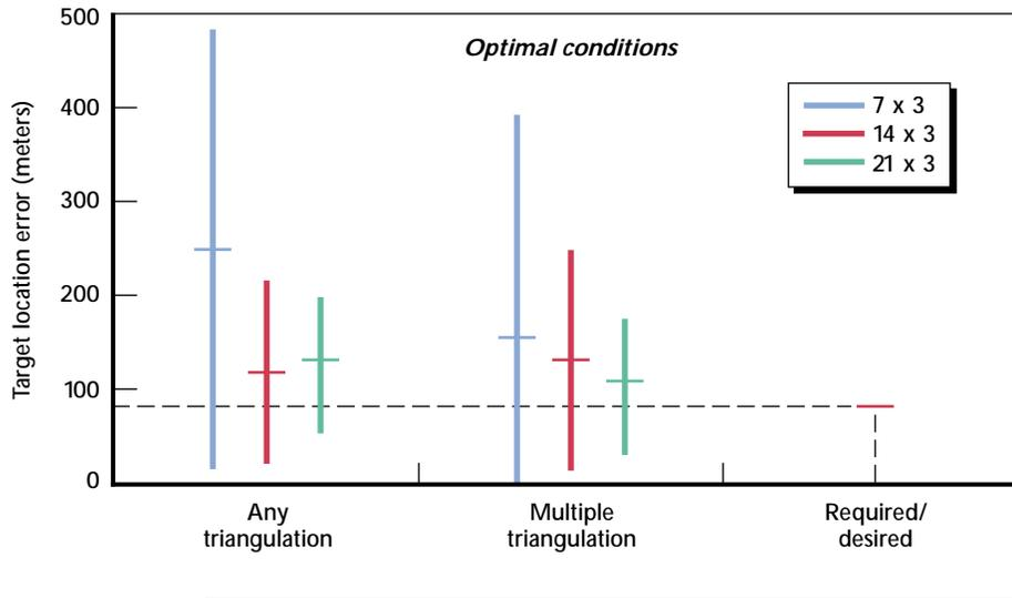
Figure 3.15—Effect of Increasing the Number of ADAS Sensors on Target Location Errors
