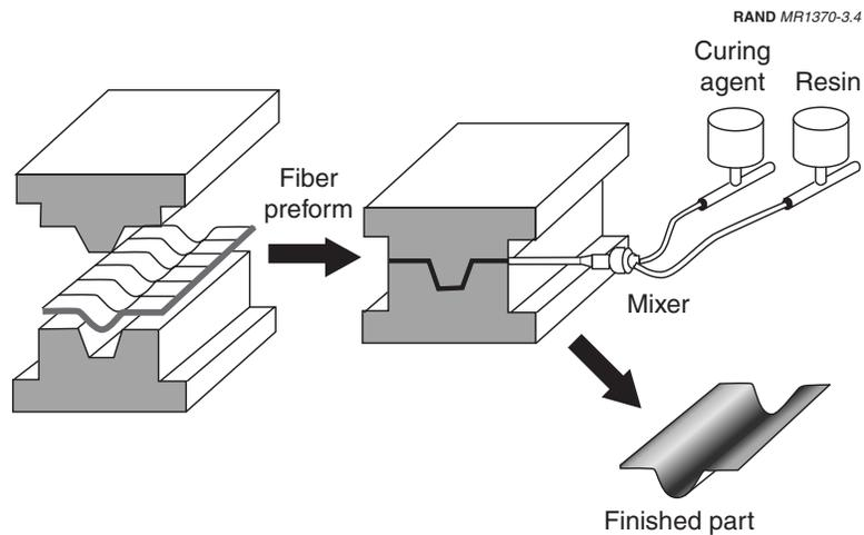
Figure 3.4—RTM Process
