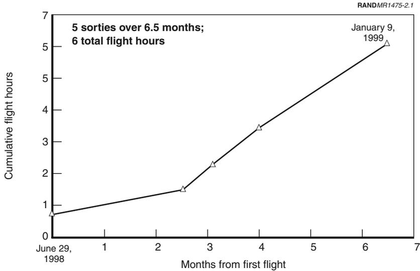
**Figure 2.1—DarkStar Air Vehicle 2 ACTD Flight Test Program**
