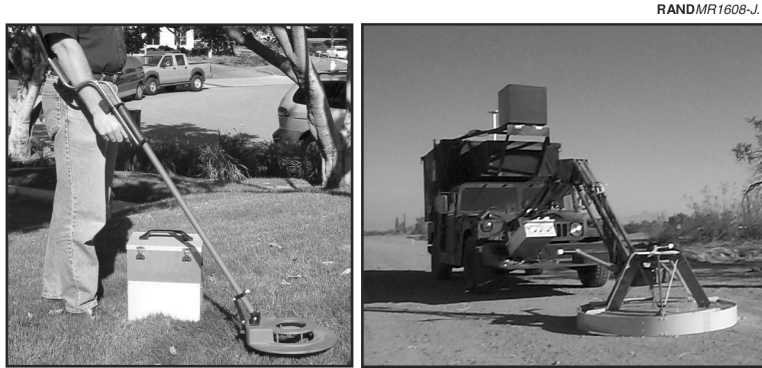
Figure J.1—Present Configuration of the Man-Portable (left) and Vehicle-Mounted NQR Systems (right)
