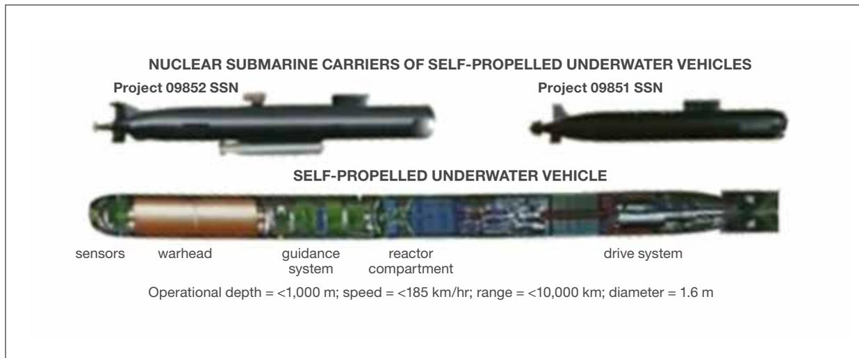
The “Oceanic Multipurpose System Status-6,” shaped like an enormous torpedo and powered by a compact nuclear reactor, would overcome enemy defenses through a combination of speed and range that would enable it to outrun almost anything in the ocean.
