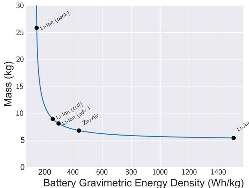
NOTE: The average energy densities of lithium ion (package and battery only) and expected densities of advanced battery chemistries (zinc-air and lithium-air) are overlaid. Li-Ion = lithium ion. Zn/Air = zinc-air. Li-Air = lithium air.
