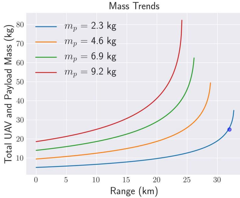
NOTE: The blue dot marks the published range and mass figures for the Amazon Prime Air Drone (as of 2016) with a 10-mile (16.1-km) operating radius or 20-mile (32.2-km) range and a 5-lb (2.3-kg) payload capacity (Amazon, undated).  $m_p$  = mission payload.
