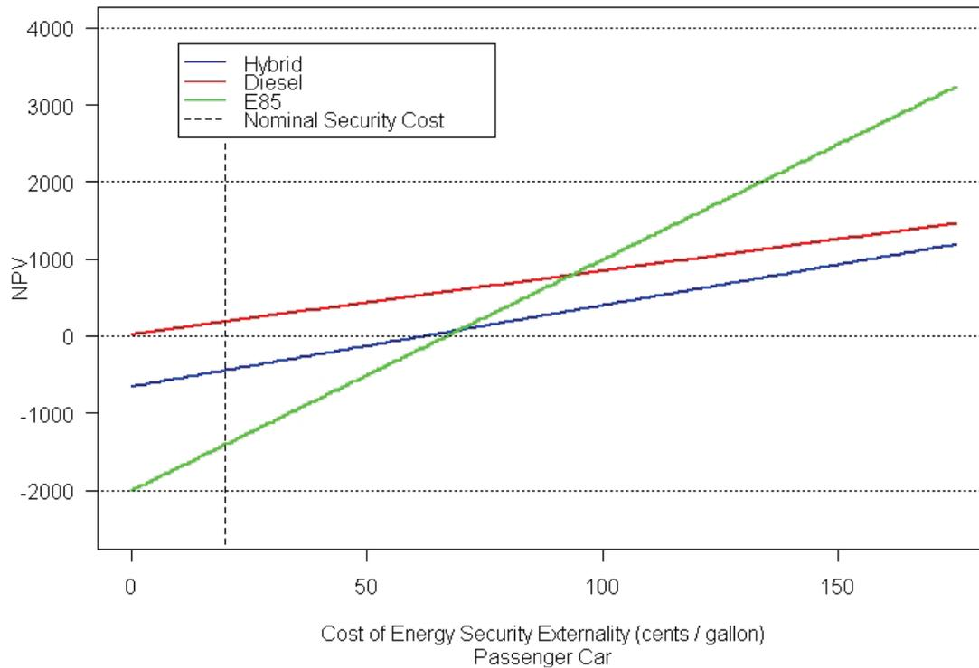
Figure 3 shows that the energy-security externality can significantly impact the results for E85. At a value of \$0.67 per gallon, E-85 has a positive NPV. With an external cost of \$0.94 per gallon, E85 NPV exceeds the two other technologies. These externality costs exceed most estimates of this value, but not all (Leiby, 2007). The figure also shows that, even with externality costs approaching \$2 per gallon, hybrids do not gain an advantage over diesel.
