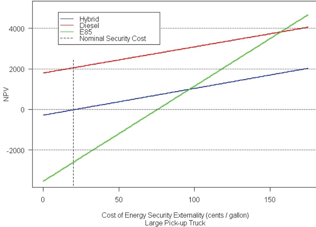
Again, Figure E-4 shows a similar result. The externality costs for oil consumption must now exceed \$0.76 per gallon for E85 to have a positive result and be greater than \$1.57 per gallon to make E85 the best option.
