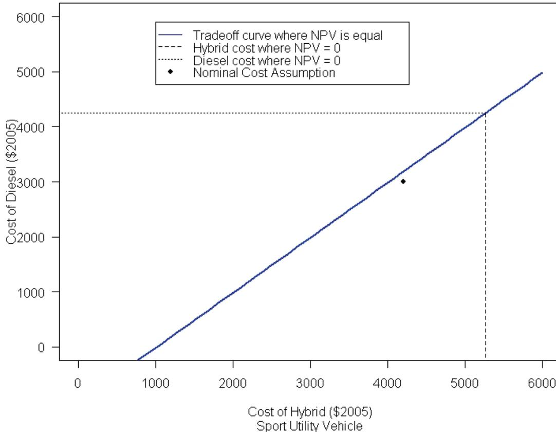
The point plotted on the graph shows the nominal cost assumptions. In this case, NPV for both technologies is positive and diesel is slightly greater. Both NPV exceed \$1,000.
