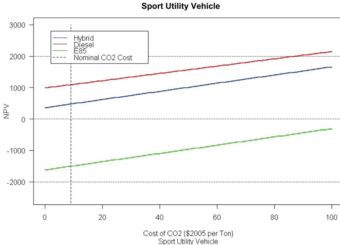
The graph shows that increasing the cost of greenhouse gas emissions improves NPV for each technology. Even at large cost values for this externality, E85 NPV does not become positive, and hybrid NPV does not exceed diesels. Figure E-2 shows the results for large pickup trucks.
