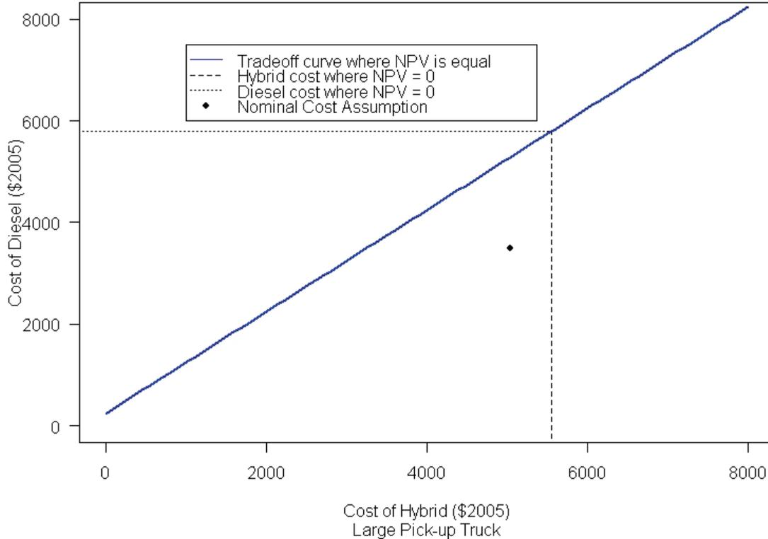
Figure D-2 shows that advanced diesel technology is more strongly favored over the hybrid for large pickup trucks. Hybrids still have positive NPV though.
