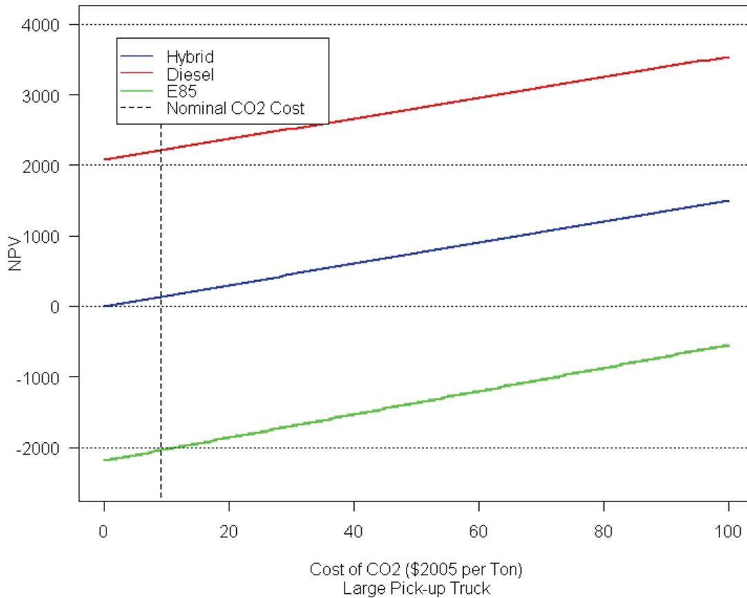
Similar to the case with SUVs, the greenhouse gas externality improves NPV for each technology. But even large values do not offset the higher fuel costs of E85 or improve the relative position of hybrids.
